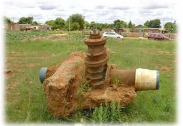
Isolating valve which had to be replaced after continuous opening and closing
